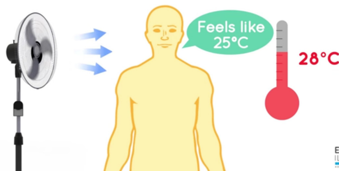
Fig. 3. Info-graphics from the Active Cooling narrative video: a) demonstration of how air movement from a fan will reduce the apparent temperature in a room; b) combined use of the air conditioner and fan can significantly reduce electricity consumption in summer.
